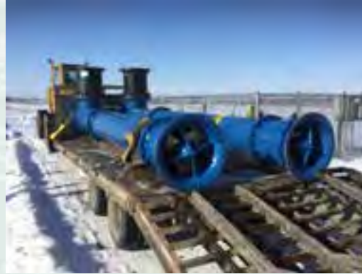
Pumps: 20,000 gpm capacity
